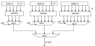
Fig5: Block Diagram of PE Unit
