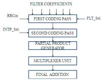
Fig 2: Data Flow Diagram Of CG Block
