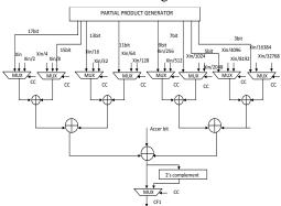
Fig 4: Multiplexer Unit and Final addition unit
