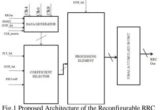
Fig.1 Proposed Architecture of the Reconfigurable RRC Filter
